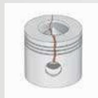
Kolbenbruch in der Kolbenbolzennabe
